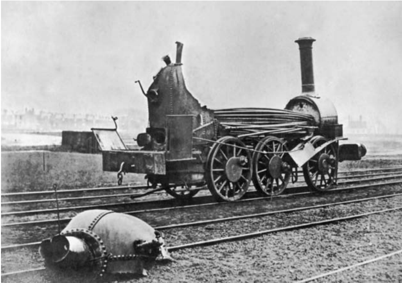
Figure 14.15 Boiler explosion about 1850 – vessel instrumentation scarcely in use at that time 13) .
