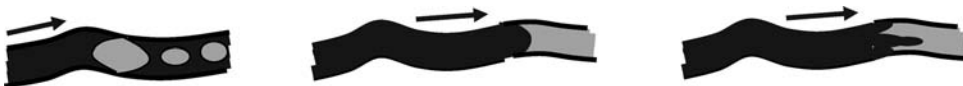
Figure 7.12 Flooding mechanisms according to the wetting behavior. P_i < P_d . (a) Water wet: imbibition, P_i . (b) Oil wet: drainage, P_d . (c) Fingering.
