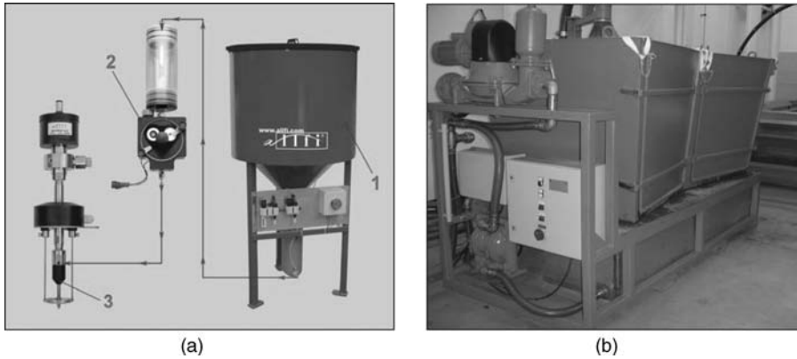
Figure 11.17 (a) Typical industrial abrasive feeding system (source: Allfi AG). (b) Sludge removal system (source: Metallbau Müller GmbH).
