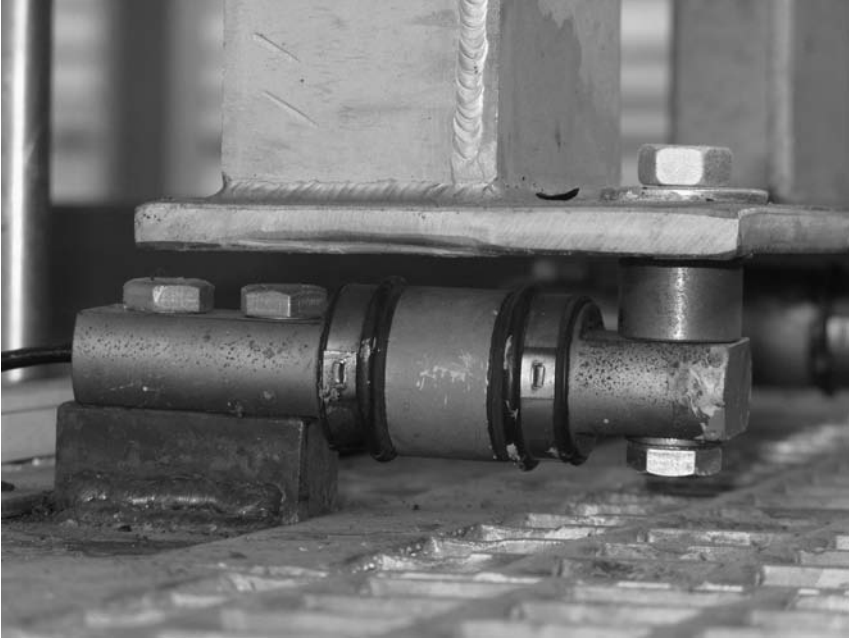
Figure 14.8 Robust level determination in high-pressure tank using a load cell.
