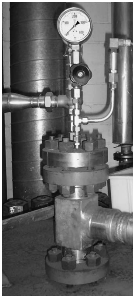
Figure 14.1 Instrumentation of high-pressure vessel (MAWP 32.5 MPa).
